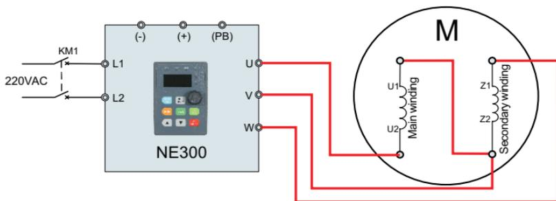
Figure 3-22 Reverse wiring between NE300 (> 0.75kW) and motor
