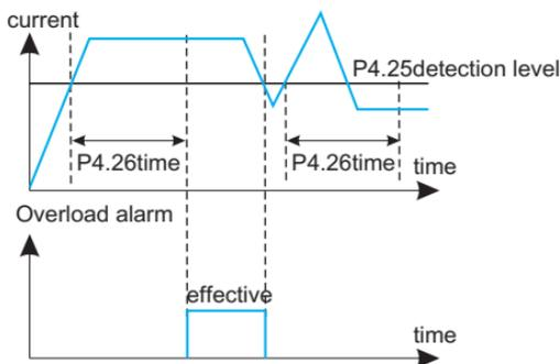
Fig.6-27 overload alarm
