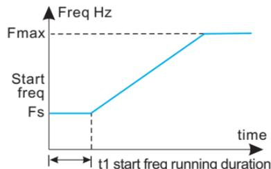
Fig.6-10 Start freq. and running duration
