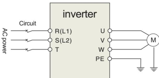
Figure 3-3 Main circuit wiring
