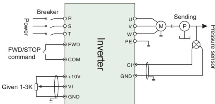
Figure 6-30 Built-in PI simulation feedback control system diagram
