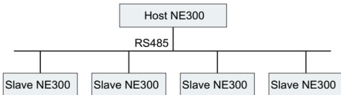
Fig9-2 The networking of multi-machine interaction
