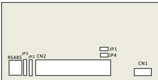
Figure 3-5 Position of terminals and jumpers on control
