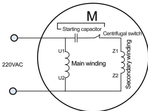
Figure 3-15 Starting mode: Internal wiring of motor with single capacitor
