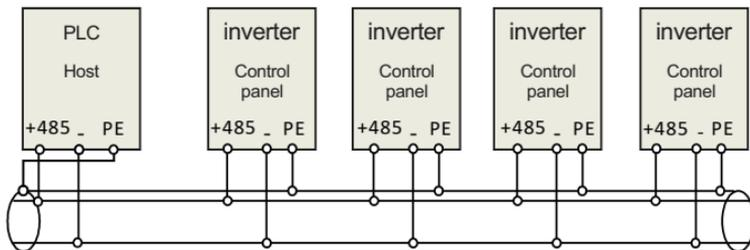
Figure 3-11 PLC communication with multi inverters
