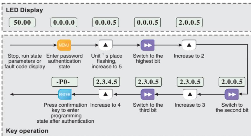
Figure 4-10 Example of password authentication operation
