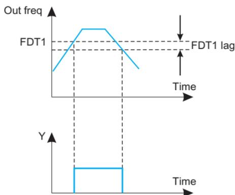
Fig.6-25 freq level detection
