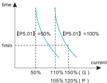
Fig. 6-30 Thermal relay protection
