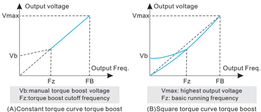
Fig.6-3 Torque boost
