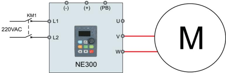
Figure 3-23 Wiring between NE300 (<=0.75Kw) and motor
