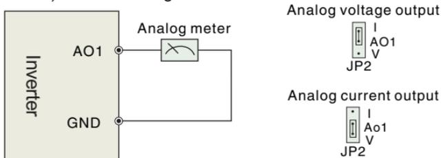
Figure 3-9 Analog output terminal wiring
