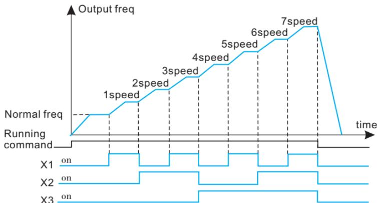
Fig 6-16 multi-stage speed running
