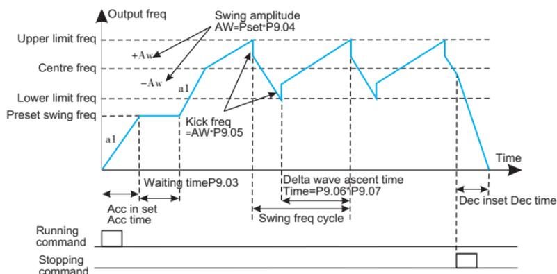
Fig.6-38 Swing frequency running
