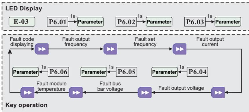
Figure 4-11 Example of inquiring fault related parameter
