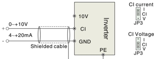
Figure 3-8 CI terminal wiring
