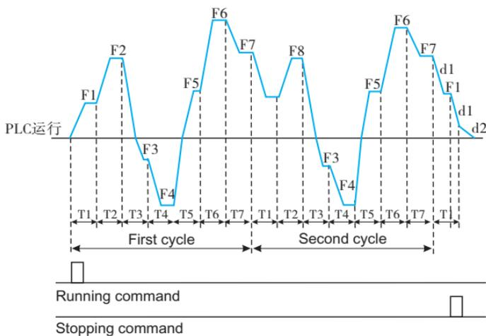
Fig.6-36 PLC continuous cycle
