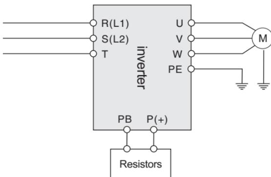
Figure 2-10 The wire connection of braking resistors
