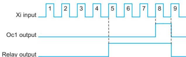
Fig.6-26 set counts given and specified counts given
