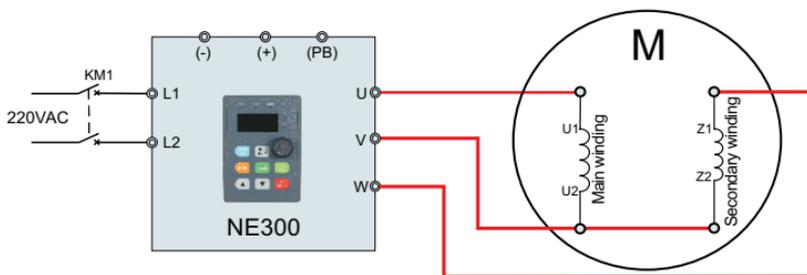
Figure 3-21 Forward wiring between NE300 (> 0.75kW) and motor
