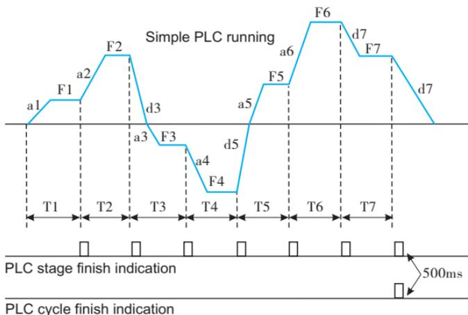
Fig.6-33 simple PLC running
