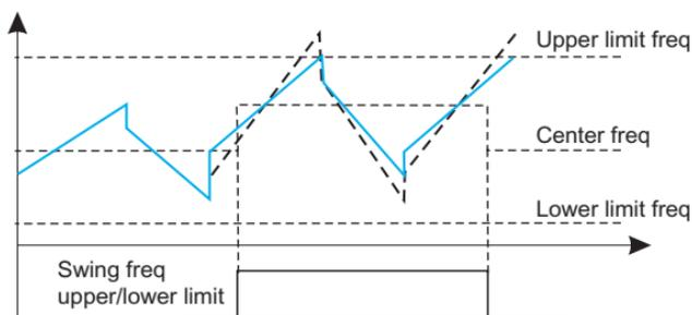
Fig.6-23 swing freq. upper/lower limit
