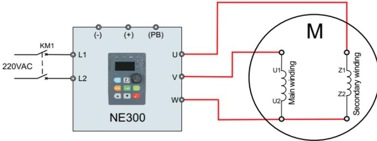
Figure 3-19 Forward wiring between NE300 (<=0.75Kw) and motor
