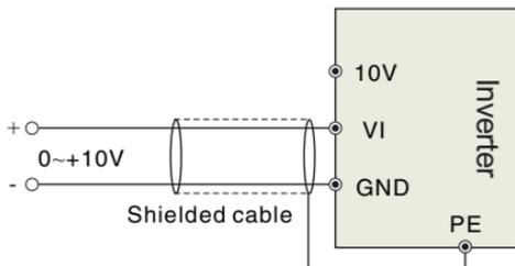
Figure 3-7 VI terminal wiring
