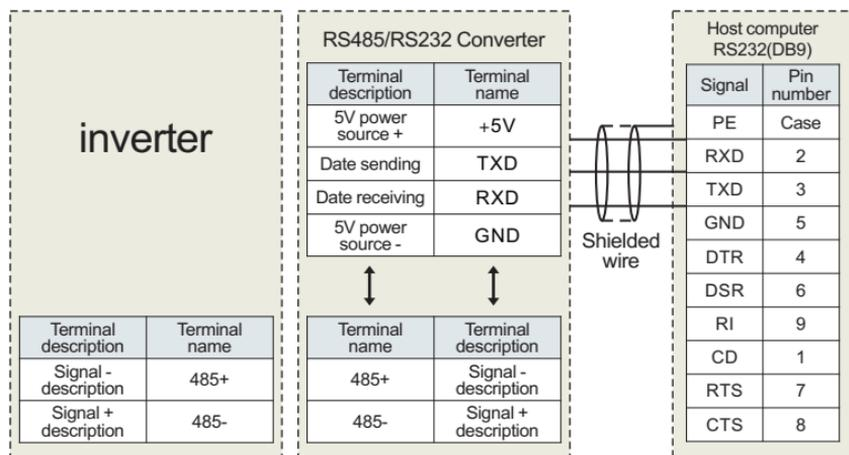
Figure 3-10 RS485-(RS485/232)-RS232 communication wiring
