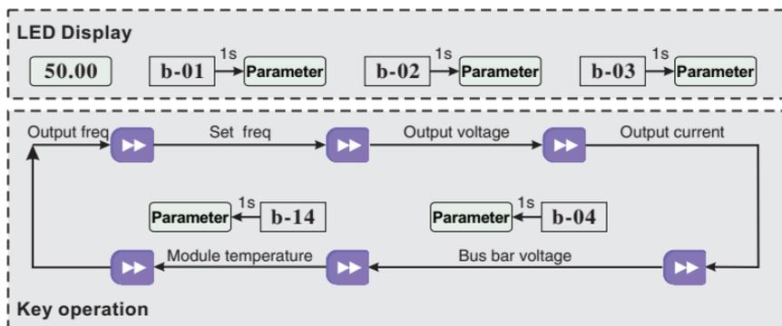
Figure 4-7 Operation to display monitoring parameter
