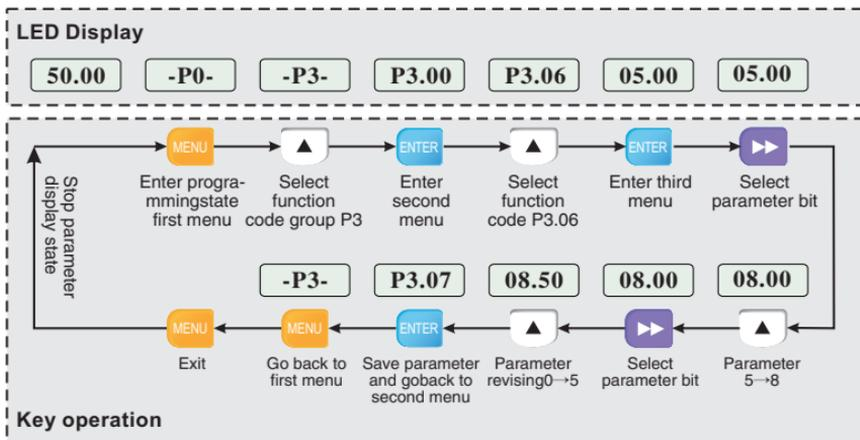
Figure 4-8 Example of function code parameter setting
