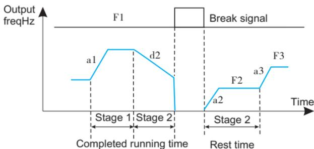
a1: Acc time of stage 1    a2: Acc time of stage 2    a3: Acc time of stage 3
