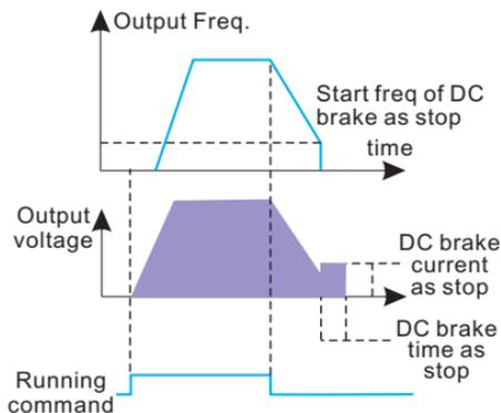
Fig.6-12 DC stop and DC brake
