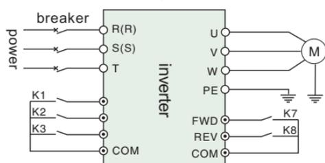
Fig.6-17 wiring diagram of multi-stage speed running
