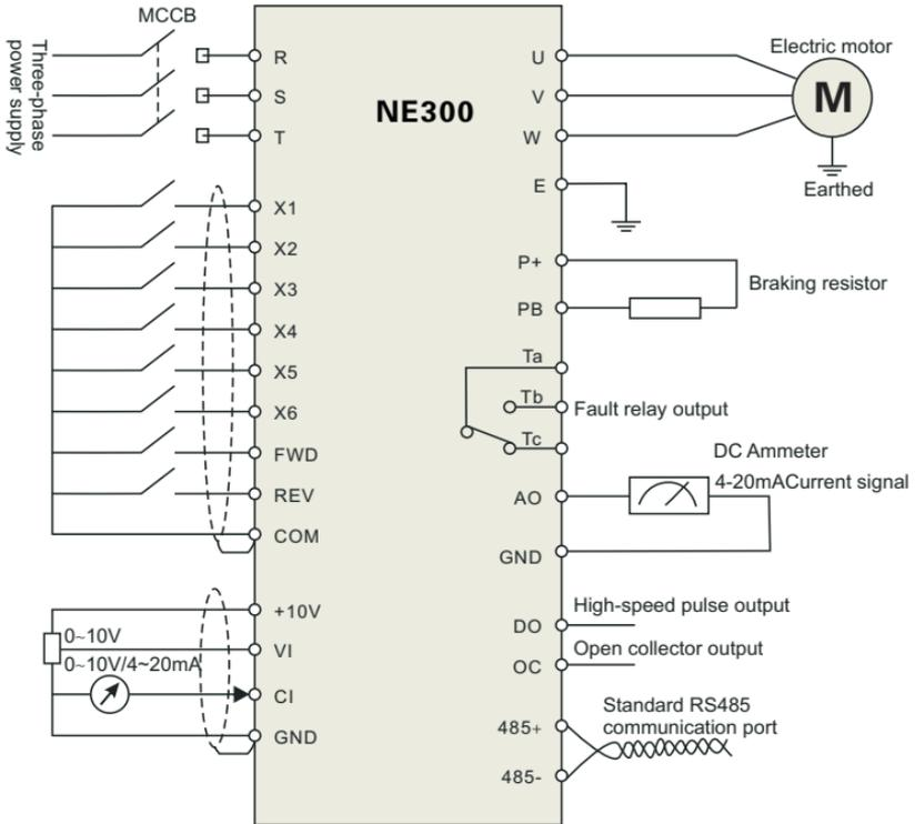
Figure 3-4 Basic Wiring Diagram
