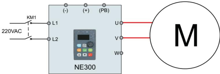
Figure 3-24 Wiring between NE300 (<=0.75Kw) and motor
