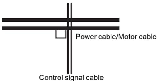
Figure 3-14 System wiring requirements
