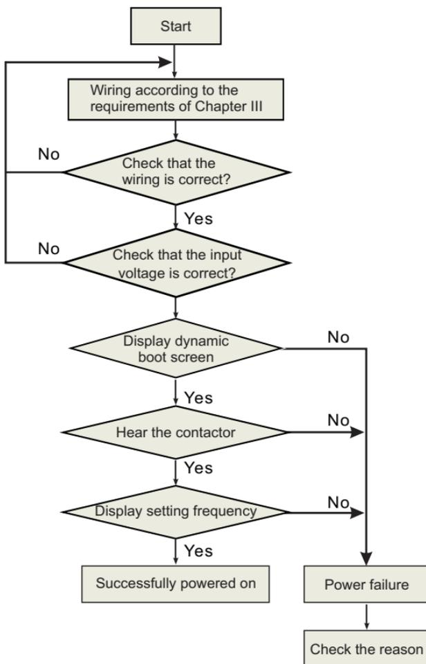
Figure 4-1 Inverter first power applied operation
