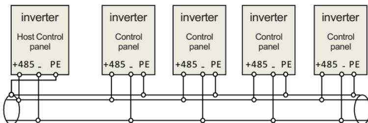
Figure 3-12 Multi inverters communication
