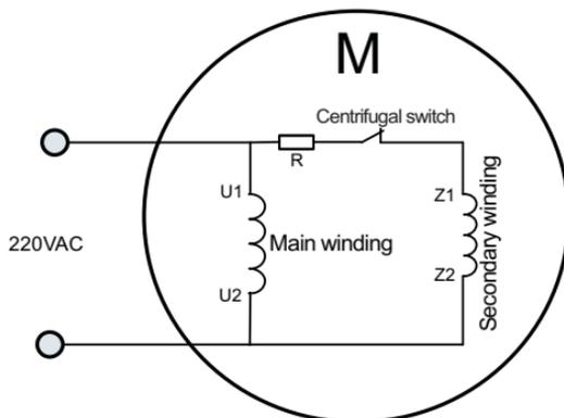
Figure 3-17 Resistor starting mode: Internal wiring of motor
