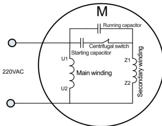
Figure 3-16 Internal wiring of motor with double capacitors
