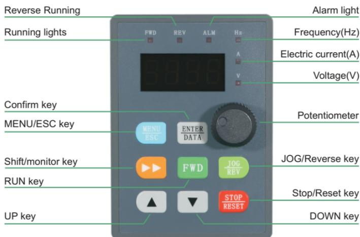
Figure 4-3 Control panel diagram
