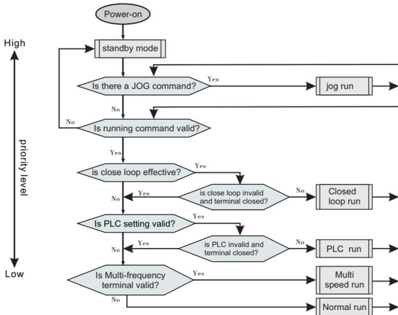
Figure 4-2 Running mode logic diagram
