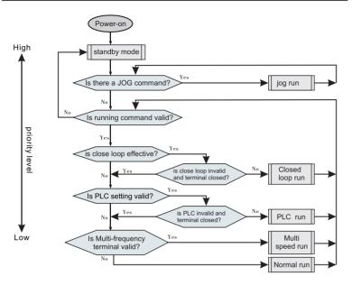
Figure 4-2 Running mode logic diagram
