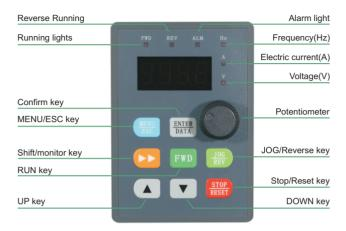
Figure 4-3 Control panel diagram
