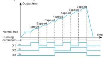
Fig 6-16 multi-stage speed running
