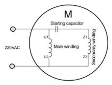
Figure 3-14 Operation mode: Internal wiring of motor with single capacitor
