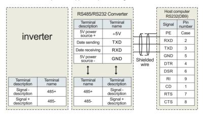
Figure 3-10 RS485-(RS485/232)-RS232 communication wiring
