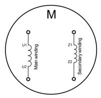
Figure 3-18 Main and secondary winding of motor (After removing the capacitors)
