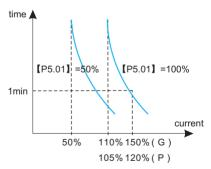
Fig. 6-30 Thermal relay protection
