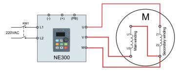
Figure 3-20 Reverse wiring between NE300 (<=0.75Kw) and motor
