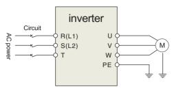
Figure 3-3 Main circuit wiring
