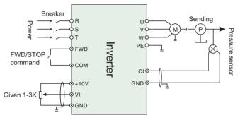
Figure 6-30 Built-in PI simulation feedback control system diagram
