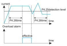
Fig.6-27 overload alarm
