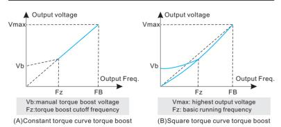
Fig.6-3 Torque boost
