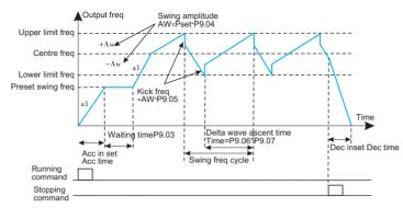
Fig.6-38 Swing frequency running
