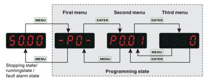
Figure 4-6 Control panel programming state
