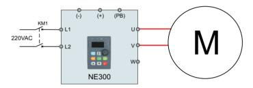
Figure 3-24 Wiring between NE300 (<=0.75Kw) and motor
