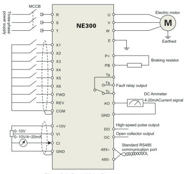
Figure 3-4 Basic Wiring Diagram
