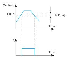
Fig.6-25 freq level detection
