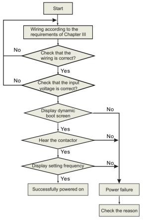
Figure 4-1 Inverter first power applied operation
