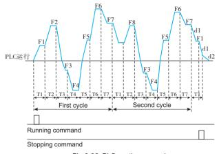
Fig.6-36 PLC continuous cycle
