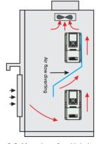
Figure 3-1 Mounting space and distance Fig
