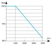
Figure 1-2 Inverter rated output current and elevation derating map
