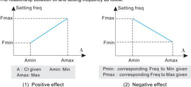
The relationship between input PULSE frequency and setting frequency is as follow.
