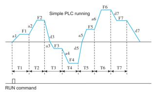
Fig.6-34 PLC stop after single cycle
