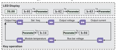
Figure 4-7 Operation to display monitoring parameter
