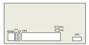
Figure 3-5 Position of terminals and jumpers on control
