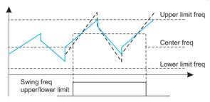
Fig.6-23 swing freq. upper/lower limit
