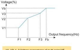
V1~V3: 1~3 Voltage percentages of multi-point V/F F1~F3:1~3 Frequency percentages of multi-point V/F Fb: Motor rated frequency
