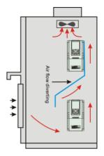
Fig.3-2 Mounting of multiple inverters
