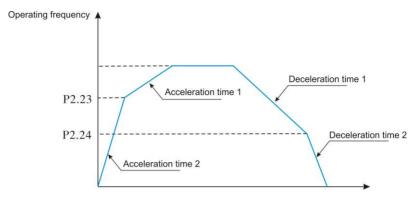
Fig. 6-12 Acceleration/deceleration switching
