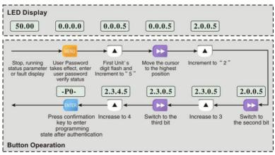
Fig.4-10 Example of entering a user password to enter a function code operation
