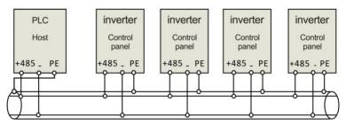
Fig. 3-12 PLC communication with multi inverters
