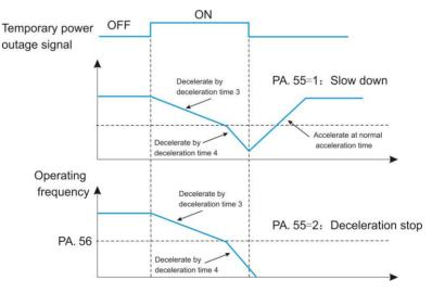
Refer to Figure 6-34 for a detailed transient stop action procedure.
