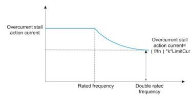
Figure 6-38 Schematic diagram of double speed over loss speed
