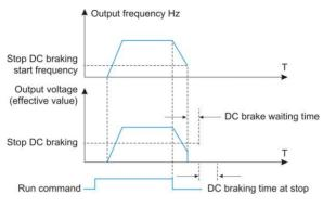
Fig. 6-02 Stop DC braking process
