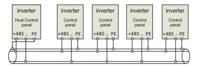
Fig. 3-13 Multi inverters communication
