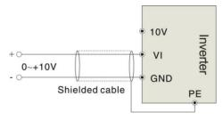
Fig. 3-7 VI terminal wiring
