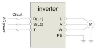
Fig. 3-3 Main circuit wiring
