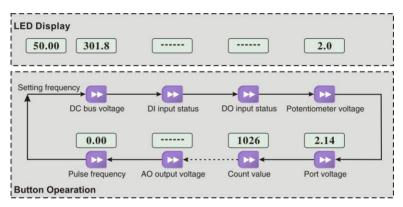
Fig.4-7 Example for running status data display operation
