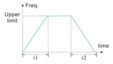
Fig. 6-03 Linear acceleration and deceleration
