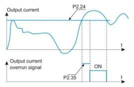
Fig. 6-14 Output current overrun detection
