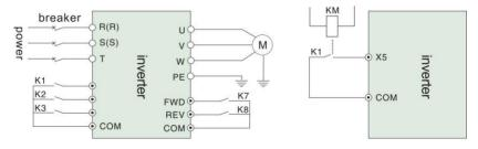
Figure 6-16 Multi-speed operation wiring diagram
