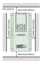
Fig.3-1 Mounting space and distance
