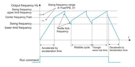
Figure 6-36 Schematic diagram of swing frequency
