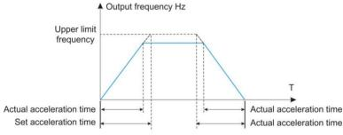
Fig. 6-1 Acceleration/Deceleration time
