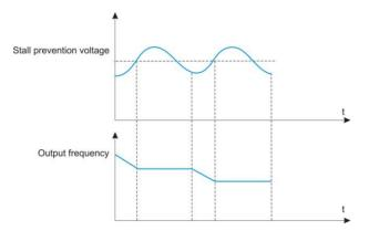
Figure 6-33 Over voltage stall function
