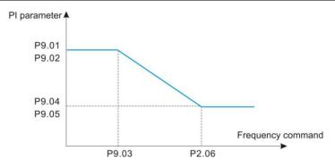
Fig. 6-32 PI parameters relationship diagram
