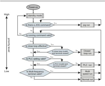
Fig. 4-2 Logical relationship diagram of inverter running status
