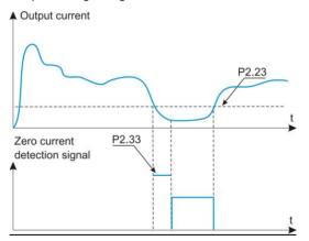
Fig. 6-13 Zero current detection
