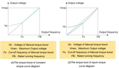
torque boost are shown in a and b of Fig.6-24.
