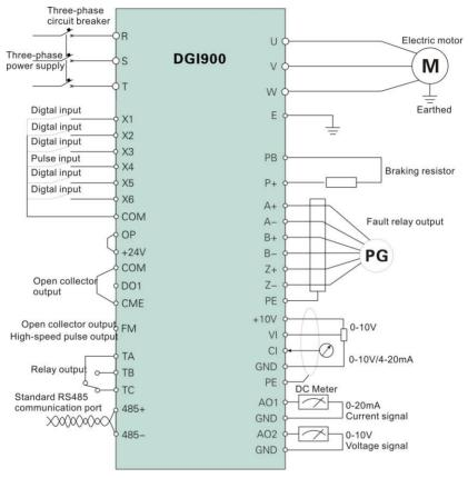
Fig. 3-4 Basic Wiring Diagram
