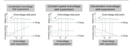
Figure 6-39 Schematic diagram of overvoltage stall action
