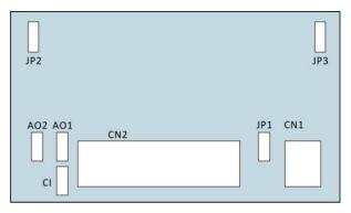
Fig. 3-5 Position of terminals and jumpers on control circuit
