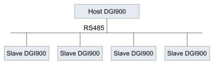
Figure 9-2 Schematic diagram of multi-machine linkage networking
