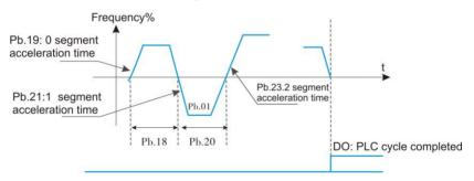
Figure 6-35 Simple PLC schematic
