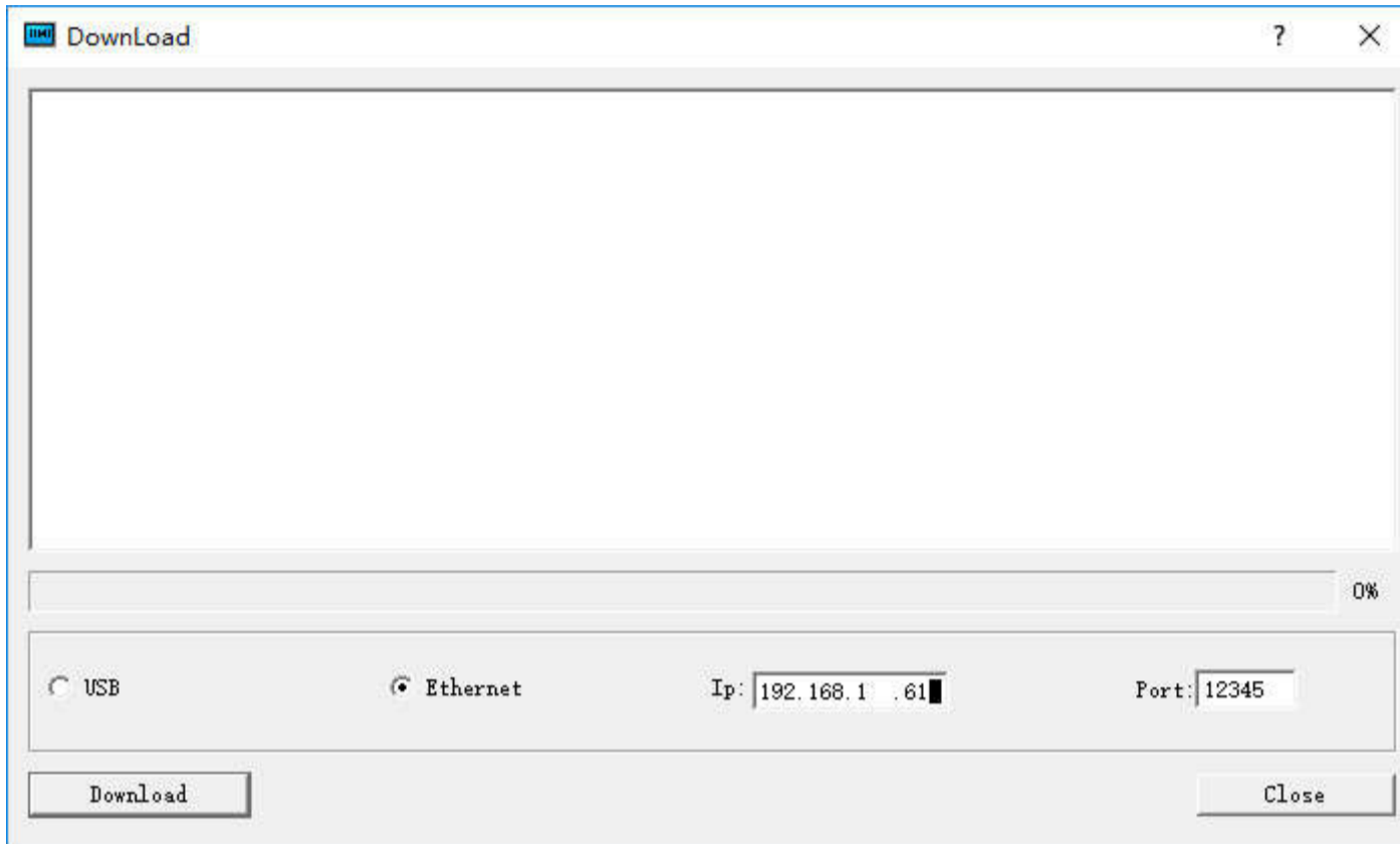
Figure 3-16 Configuration downloading through Ethernet
